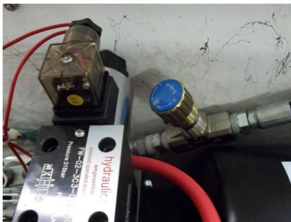
12. Use caution operating your lift during low battery voltage conditions. Although the safe 12 DC motor can survive lower voltage conditions the starter solenoid for this motor requires the full 12 volts to energize the magnetic switch to ‘clamp’ the contacts without arcing.
