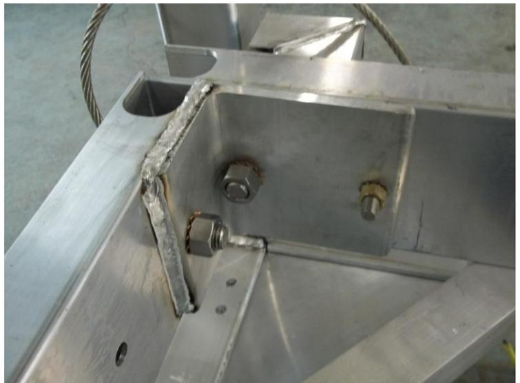
HD and a ½ brass nut on the inside hole of the rack. Do this for all 4 corners.
